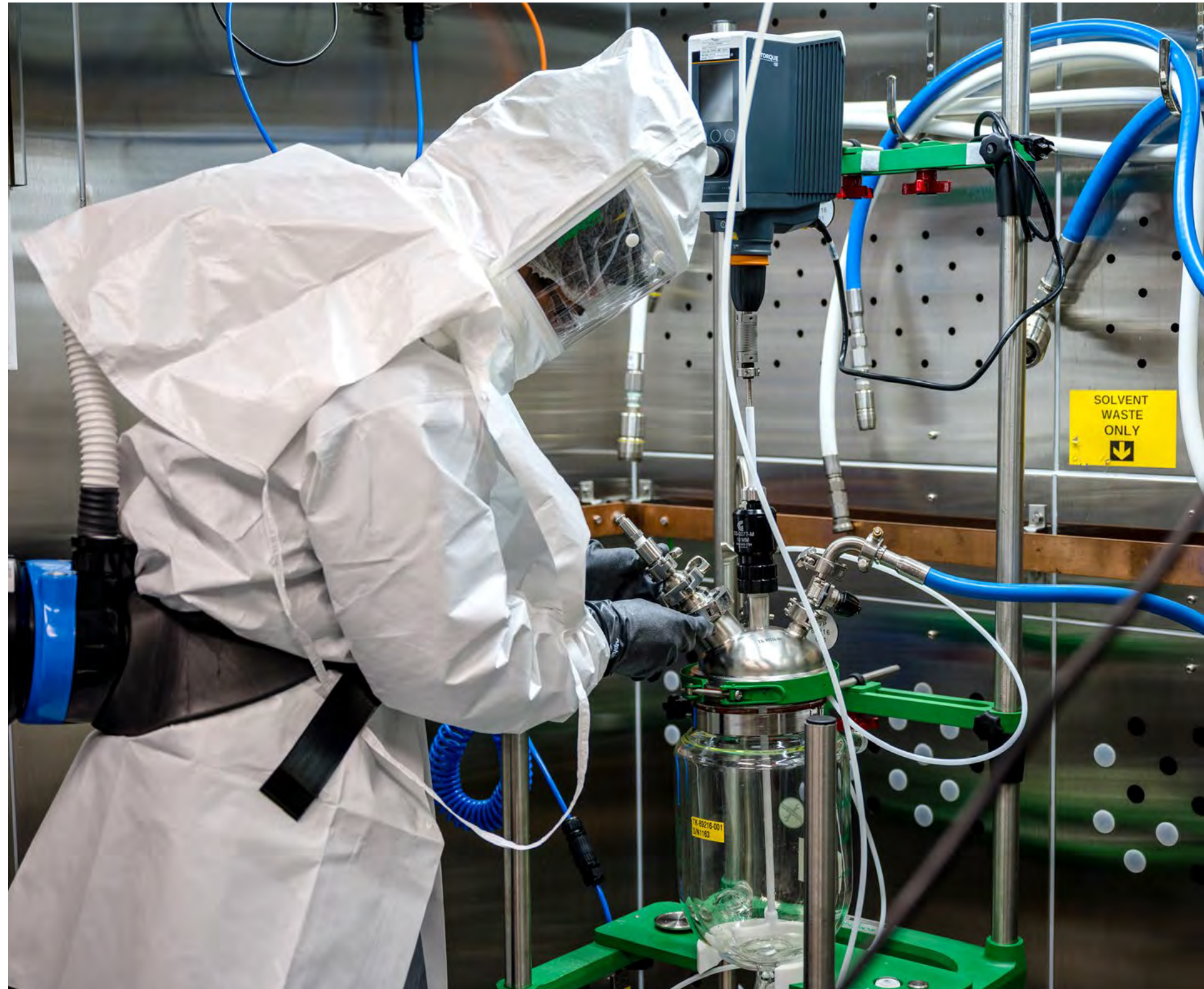
A Research Triangle Park Pharma employee wears a powered air-purifying respirator to safeguard and control exposure of solvents while working in the Oligonucleotide Synthesis Manufacturing suite.
